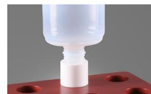
Closeup view of CleanClever in heating well
